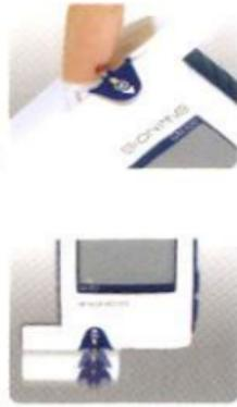
1. Insert the strip into the glucose meter and wait for the information on the top of the strip to appear.
